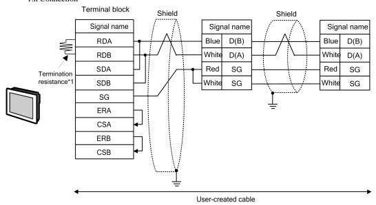
\*1 The resistance in the Display is used as the termination resistance. Set the value of the DIP Switch on the rear of the Display as shown in the table below.
