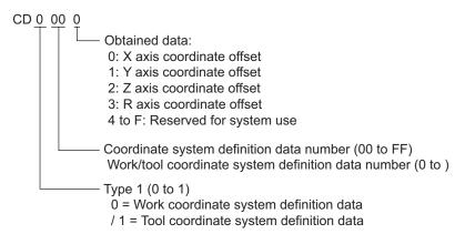
\*25 The device descriptions of simple interference check zone data are shown below.
