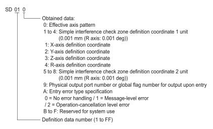
\*26 The device descriptions of Scara absolute coordinate movement are shown below.
