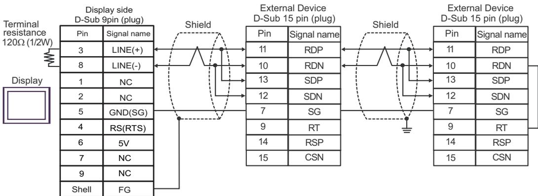
**IMPORTANT** • The 5V output (Pin #6) on the Display is the power for the Siemens AG's PROFIBUS connector. Do not use it for other devices.
