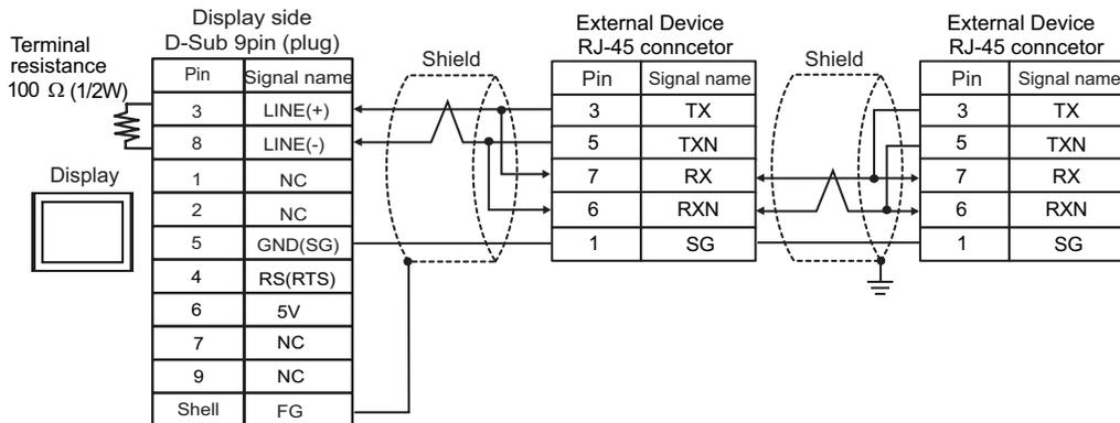
**IMPORTANT** • The 5V output (Pin #6) on the Display is the power for the Siemens AG's PROFIBUS connector. Do not use it for other devices.
