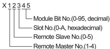
(Example) Remote External Input Remote Master No.1, Remote Slave No.2, Slot No.3, Internal Module Word No.4
