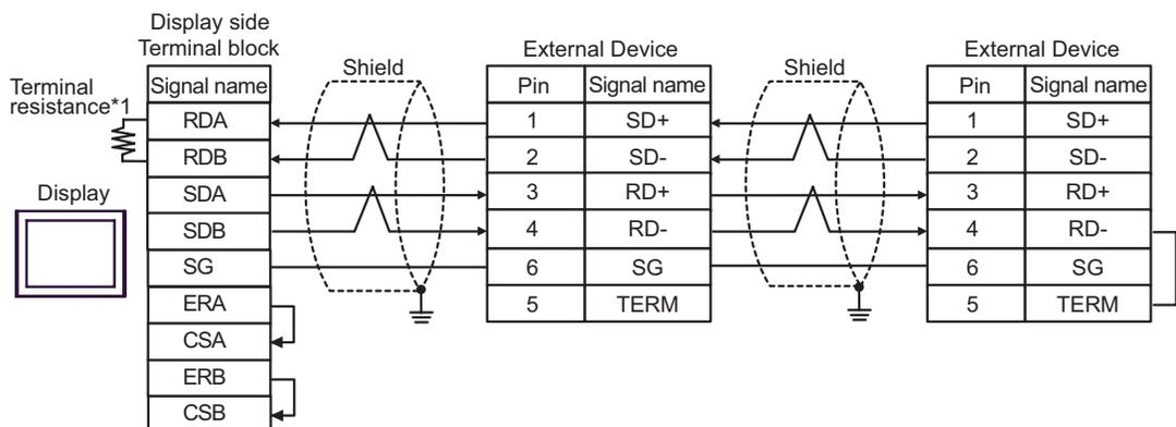
\*1 The resistance in the Display is used as the termination resistance. Set the value of the DIP Switch on the rear of the Display as shown in the table below.
