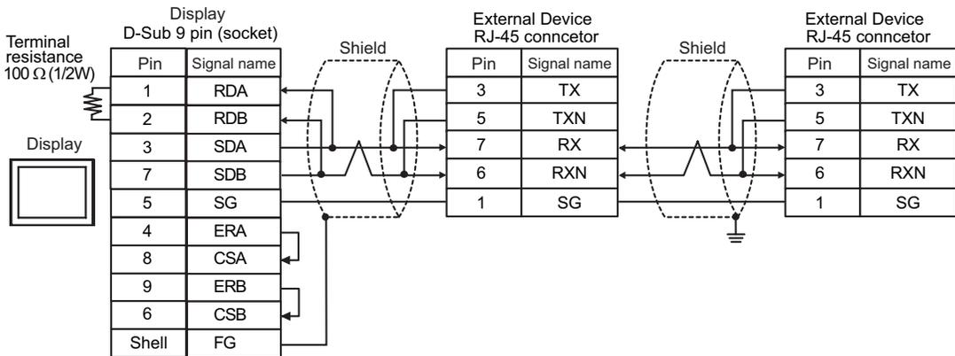
**NOTE** • Please turn on the DIP Switch 1 to enable build-in resistance(100Ω) on the remotest External Device side.
