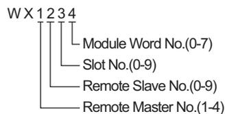
**NOTE** • Available type and range of device vary depending on CPU. Be sure to check them in each CPU manual before using.
