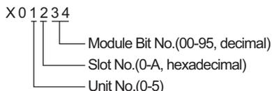
(Example) External input unit No.1, Slot No.2, Internal Module Word No.3
