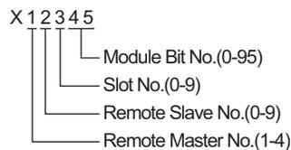
(Example) Remote External Input Remote Master No.1, Remote Slave No.2, Slot No.3, Internal Module Word No.4
