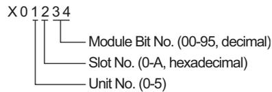
(Example) External input unit No.1, Slot No.2, Internal Module Word No.34
