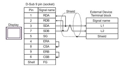
D-Sub 9 pin (socket) Pin Signal name Shield External Device Terminal block External Device Terminal block RDA 2 RDB Signal name Signal name Display 3 SDA L1 L1 SDB L2 L2 7 5 SG Shield Shield 4 **ERA** 8 CSA 9 ERB CSB 6 FG Shell
