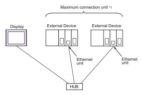
\*1 You can connect up to 32 units of External Device for UDP, and 16 units of External Device for TCP at the same time.
