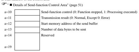
A send buffer temporarily stores data that will be sent to the SIO. You can then run the Send command to send the data in the buffer from the SIO.
