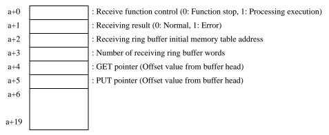
Receiving buffer that stores receive data is defined by using this Receive Function Control Area. In general, Display sets this definition immediately after the start.
