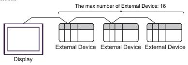
• 1:n connection (For JU series with temperature controller feature)
