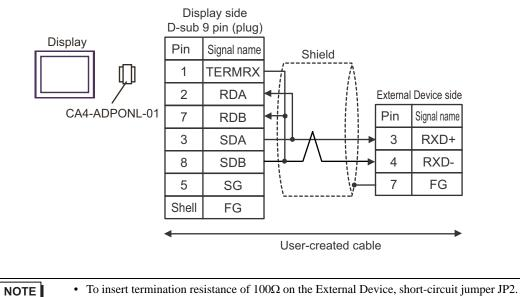
• For the External Device connector, use the XH connector (XHP-7) by J.S.T. Mfg.
