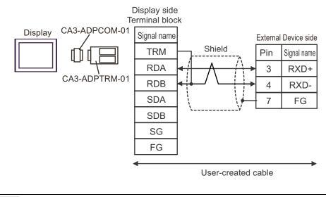
• To insert termination resistance of  $100\Omega$  on the External Device, short-circuit jumper JP2.
