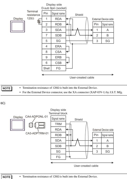
• For the External Device connector, use the XA connector (XAP-03V-1) by J.S.T. Mfg.
