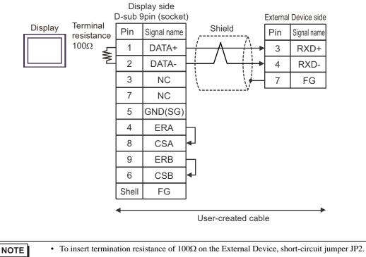
• For the External Device connector, use the XH connector (XHP-7) by J.S.T. Mfg.
