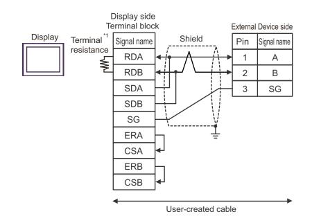
\*1 The resistance built into the Display is used as termination resistance. Please set the DIP Switch in the back of the Display as follows.
