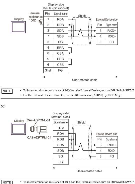
• For the External Device connector, use the XH connector (XHP-8) by J.S.T. Mfg.
