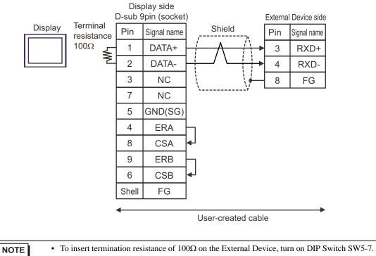
• For the External Device connector, use the XH connector (XHP-8) by J.S.T. Mfg.
