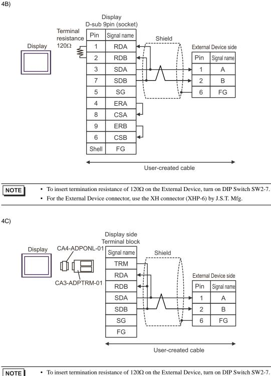
• For the External Device connector, use the XH connector (XHP-6) by J.S.T. Mfg.
