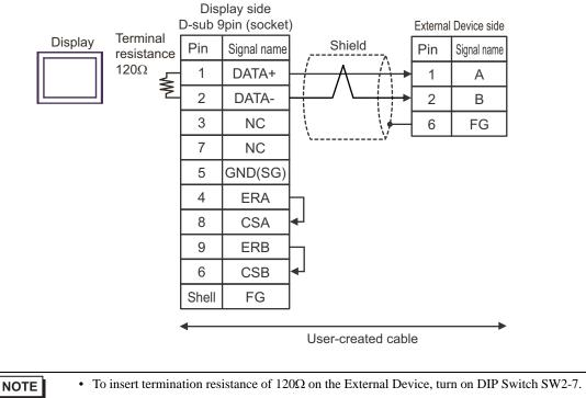
• For the External Device connector, use the XH connector (XHP-6) by J.S.T. Mfg.
