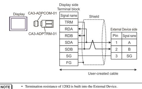
• For the External Device connector, use the XA connector (XAP-03V-1) by J.S.T. Mfg.
