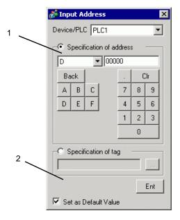
Select either [Specification of address] or [Specification of tag] to set addresses.
