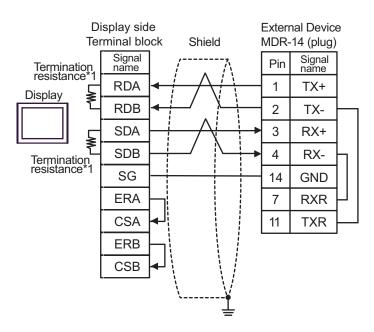
\*1 The resistance in the Display is used as the termination resistance. Set the value of the DIP Switch on the rear of the Display as shown in the table below.
