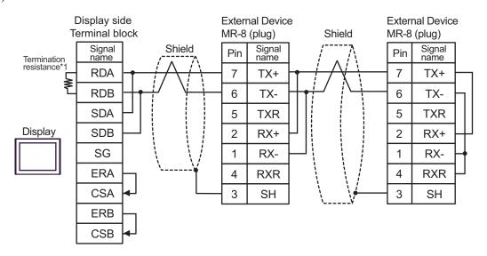
\*1 The resistance in the Display is used as the termination resistance. Set the value of the DIP Switch on the rear of the Display as shown in the table below.
