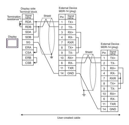
\*1 The resistance in the Display is used as the termination resistance. Set the value of the DIP Switch on the rear of the Display as shown in the table below.
