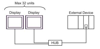
• The number of connectable Displays depends on the External Device.
