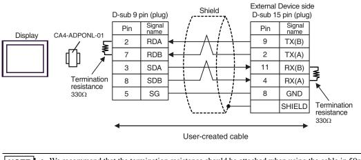
**NOTE** • We recommend that the termination resistance should be attached when using the cable in 50m or more length.
