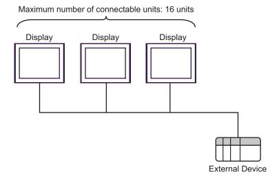
• The maximum number of connectable Displays is 16 units. However, keeping performance in consideration, the number of Displays that can be substantially used is up to 4.
