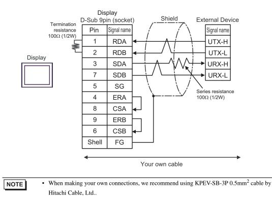
C) When using the online adapter (CA4-ADPONL-01), the connector terminal block conversion adapter (CA3-ADPTRM-01) by Pro-face and your own cable
