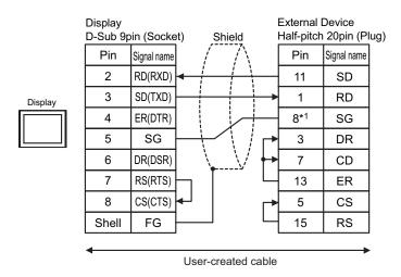
\*1 When connecting with 30i-Model A, 31i-Model A or 32i-Model A, The pin number of SG changes with ports to be used.
