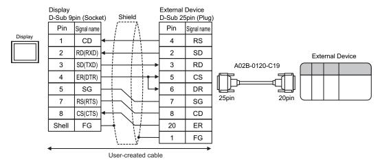
2B) Display side **External Device** Terminal block Shield D-Sub 25pin (Plug) Pin Signal name Signal name Display CD 4 RS RD(RXD) SD **External Device** 3 SD(TXD) RD A02B-0120-C19 ER(DTR) 5 CS SG 6 DR 25pin 20pin RS(RTS) SG CS(CTS) CD 20 ER 1 FG User-created cable
