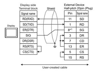
\*1 When connecting with 30i-Model A, 31i-Model A or 32i-Model A, The pin number of SG changes with ports to be used.
