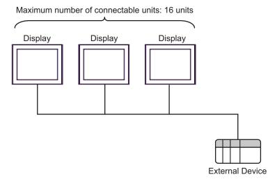
• You can connect a maximum of 16 Displays. However, for optimum performance, we recommend using a maximum of four Displays.
