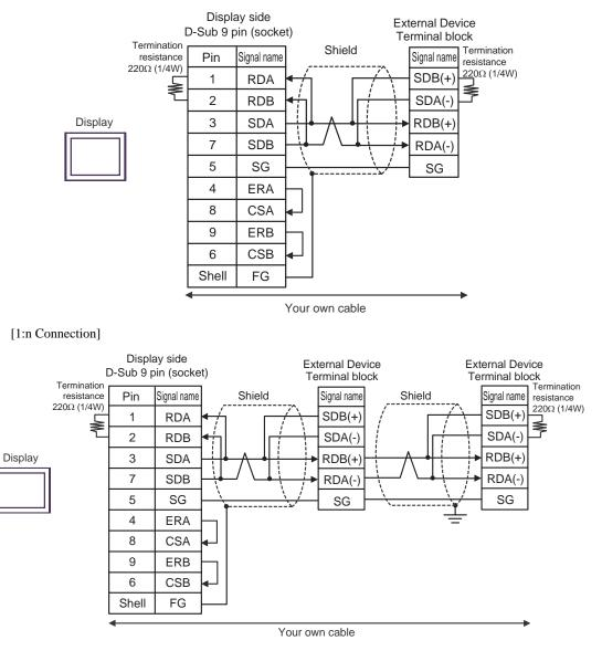
C) When using the online adapter (CA4-ADPONL-01) by Pro-face, the terminal block conversion adapter (CA3-ADPTRM-01) by Pro-face and your own cable
