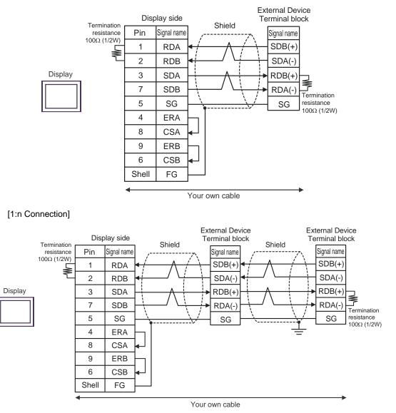
C) When using the online adapter (CA4-ADPONL-01) by Pro-face, the terminal block conversion adapter (CA3-ADPTRM-01) by Pro-face and your own cable
