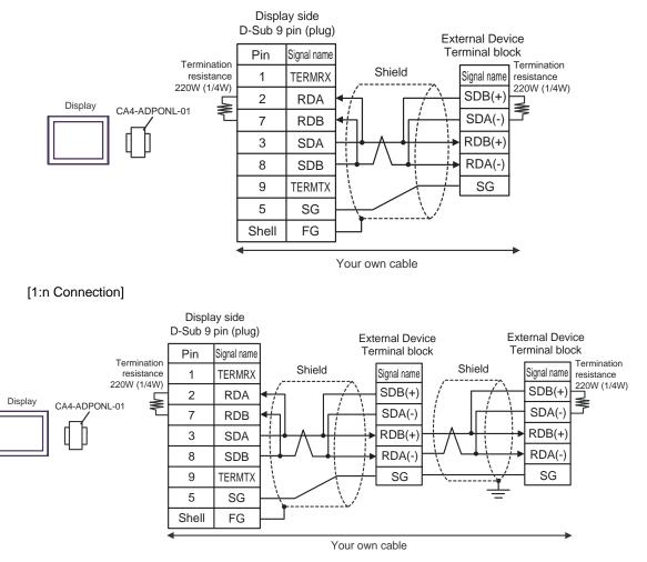
E) When using the COM port conversion adapter (CA3-ADPCOM-01), the terminal block conversion adapter
