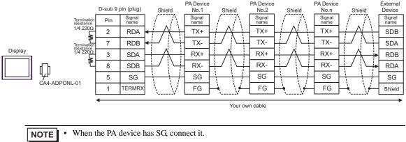
• Even if the PA device has no SG, SG connection between the Display and the External Device is necessary.
