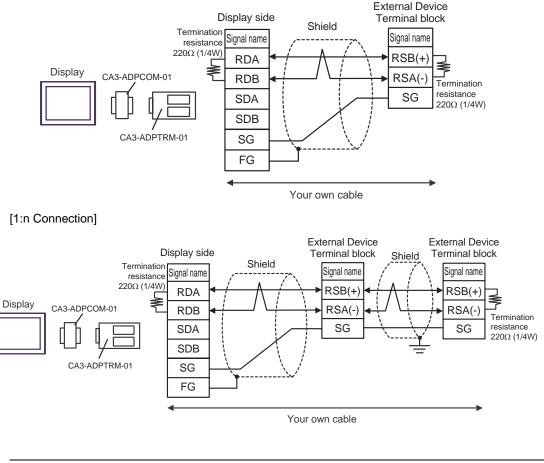
• When the display unit you use is an IPC, turn ON the DIP switch 6 to insert the termination resistance.
