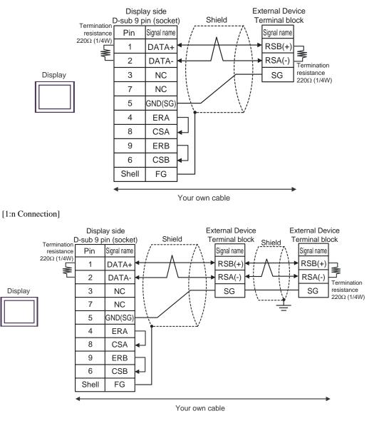
• When the display unit you use is an IPC, turn ON the DIP switch 6 to insert the termination resistance.
