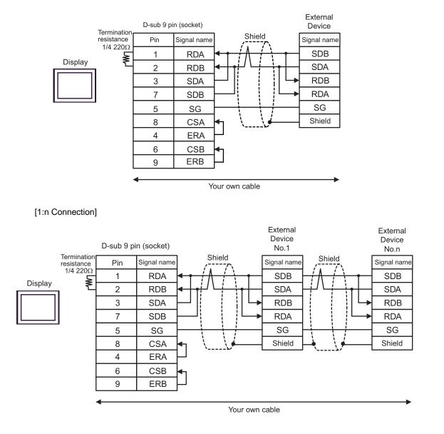
C) When using the online adapter (CA4-ADPONL-01) by Pro-face, the terminal block conversion adapter (CA3-ADPTRM-01) by Pro-face and your own cable
