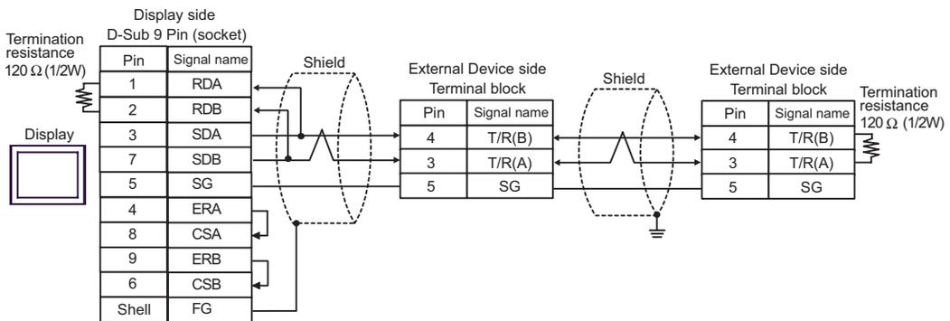
C) When using the online adapter (CA4-ADPONL-01), the terminal block conversion adapter (CA3-ADPTRM-01) by Pro-face, and a user-created cable.
