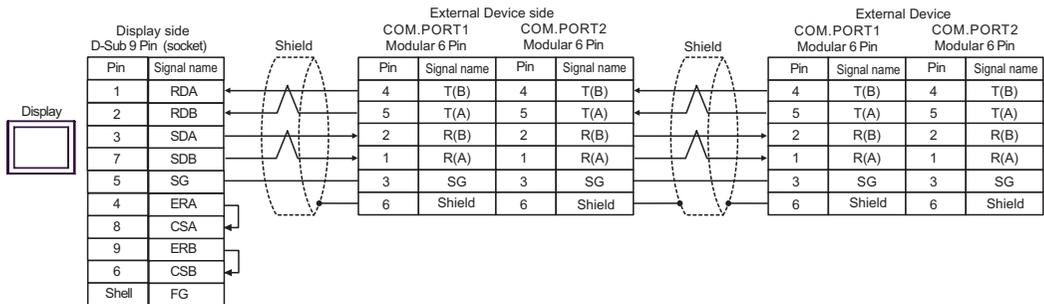
**NOTE** • Termination resistance is not necessary.
