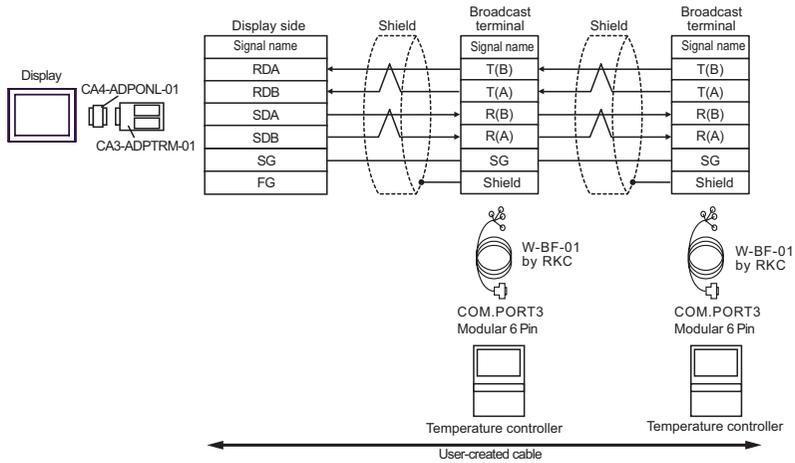
**NOTE** • Termination resistance is not necessary.
