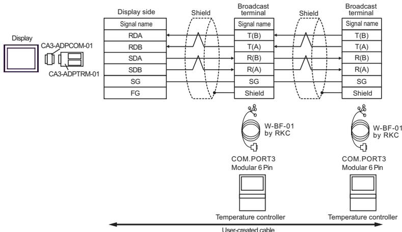
**NOTE** • Termination resistance is not necessary.
