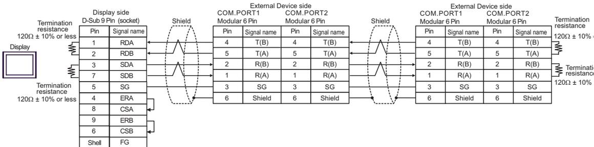
C) When using the online adapter (CA4-ADPONL-01), the terminal block conversion adapter (CA3-ADPTRM-01) by Pro-face, and a user-created cable
