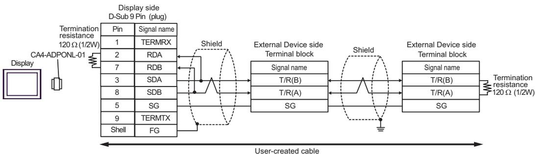
E) When using the COM port conversion adapter (CA3-ADPCOM-01), the terminal block conversion adapter (CA3-ADPTRM-01) by Pro-face, and a user-created cable
