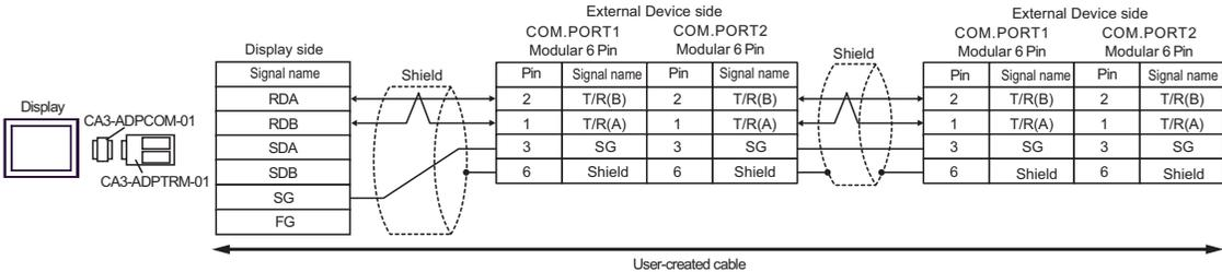
**NOTE** • Termination resistance is not necessary.
