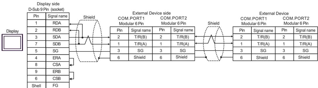
**NOTE** • Termination resistance is not necessary.
