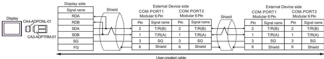
**NOTE** • Termination resistance is not necessary.
