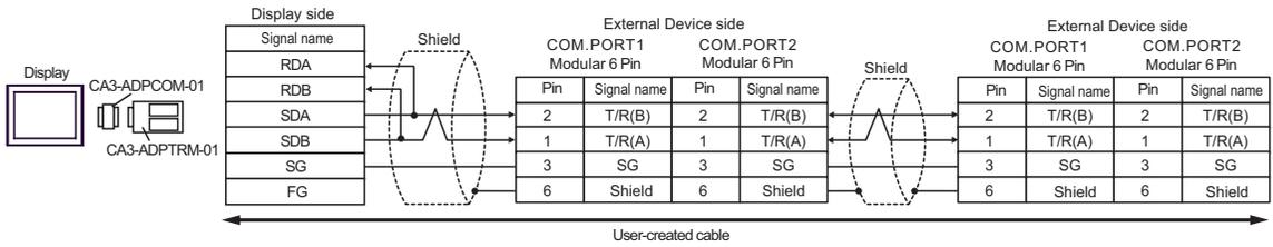
**NOTE** • Termination resistance is not necessary.
