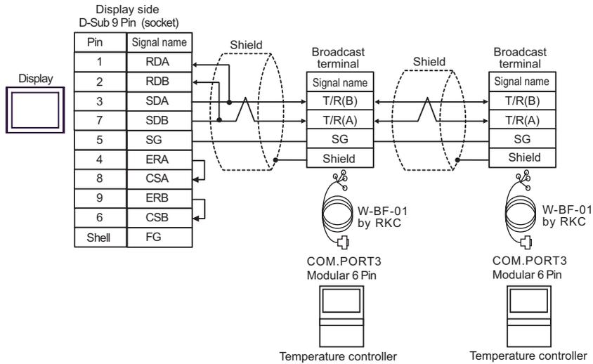
**NOTE** • Termination resistance is not necessary.
