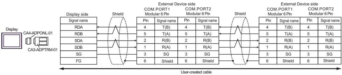
**NOTE** • Termination resistance is not necessary.
