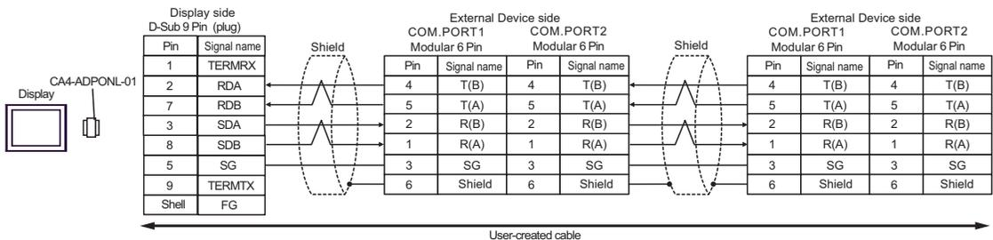
**NOTE** • Termination resistance is not necessary.
