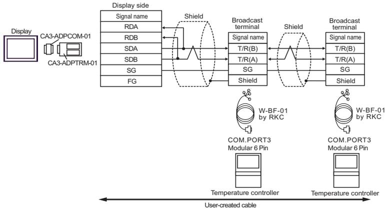
**NOTE** • Termination resistance is not necessary.
