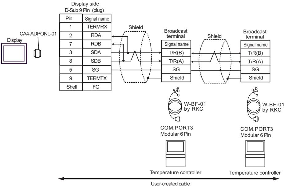
**NOTE** • Termination resistance is not necessary.
