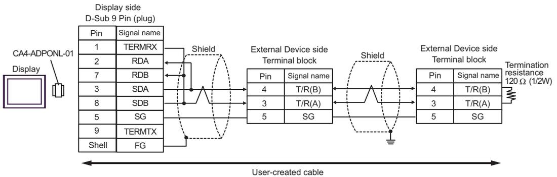
E) When using the COM port conversion adapter (CA3-ADPCOM-01), the terminal block conversion adapter (CA3-ADPTRM-01) by Pro-face, and a user-created cable.
