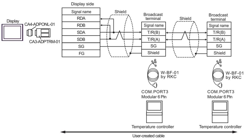
**NOTE** • Termination resistance is not necessary.
