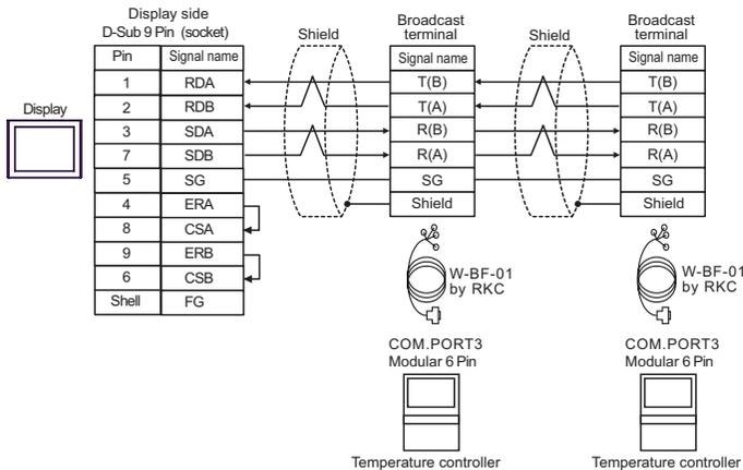
**NOTE** • Termination resistance is not necessary.
