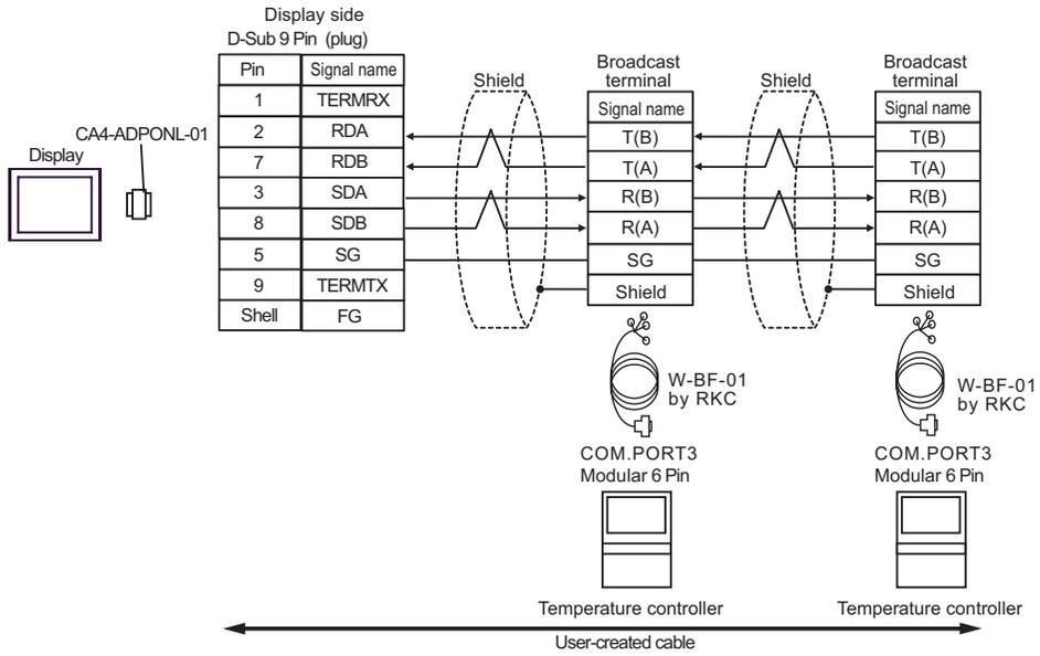
**NOTE** • Termination resistance is not necessary.
