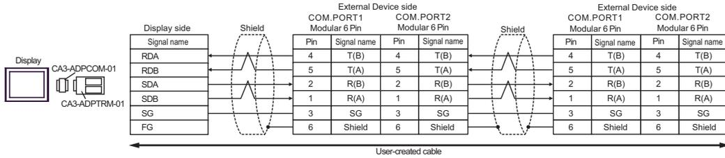
**NOTE** • Termination resistance is not necessary.
