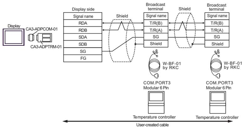
**NOTE** • Termination resistance is not necessary.
