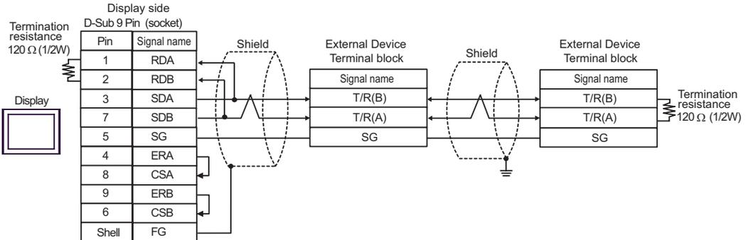
C) When using the online adapter (CA4-ADPONL-01), the terminal block conversion adapter (CA3-ADPTRM-01) by Pro-face, and a user-created cable
