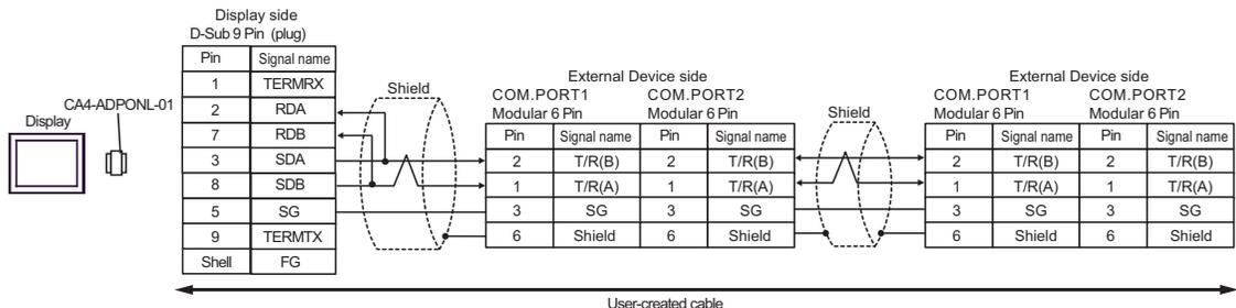
**NOTE** • Termination resistance is not necessary.
