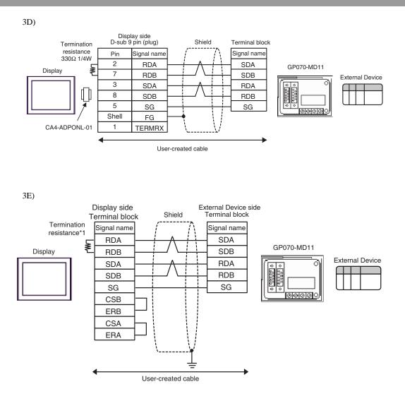
\*1 The resistance in the Display is used as the termination resistance. Set the value of the DIP Switch on the rear of the Display as shown in the table below.
