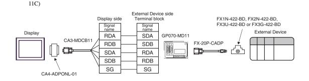
Display side D-sub 9 pin (plug) External Device side FX1N-422-BD, FX2N-422-BD, Signal Terminal block Termination FX3U-422-BD or FX3G-422-BD name resistance Signal TRMRX 1 Display External Device 330Ω 1/4W năme GP070-MD11 2 **RDA** SDA FX-20P-CADP 7 SDB **RDB ®** 3 **RDA** SDA 8 SDB **RDB** 5 SG SG CA4-ADPONL-01 Shell FG User-created cable
