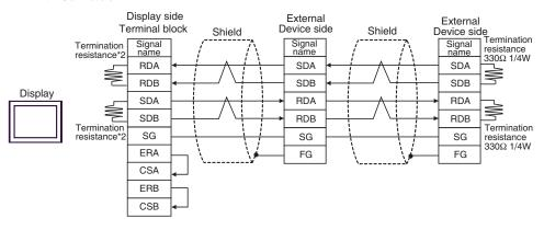
\*2 The resistance in the Display is used as the termination resistance. Set the value of the DIP Switch on the rear of the Display as shown in the table below.
