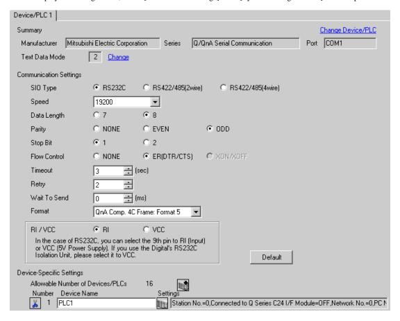
To display the setting screen, click [[[Setting]]] of External Device you want to set from [Device-Specific Settings] of [Device/PLC Settings].
