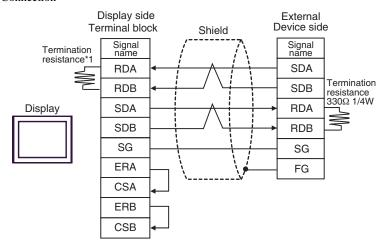
\*1 The resistance in the Display is used as the termination resistance. Set the value of the DIP Switch on the rear of the Display as shown in the table below.
