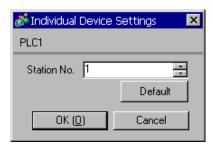
Use the ladder software (WinProladder) for communication settings. After completing the settings, reboot the External Device to enable them. Refer to your External Device manual for details.
