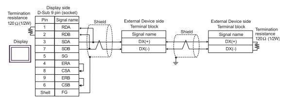
C) When using the online adapter (CA4-ADPONL-01), the terminal block conversion adapter
