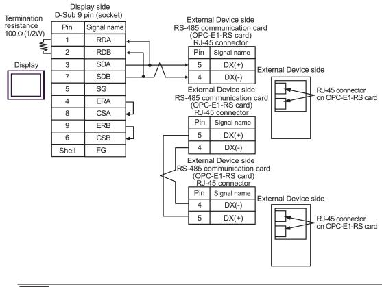
• For 1:n connection, set the termination resistance switch on the External Device located at the end to ON.
