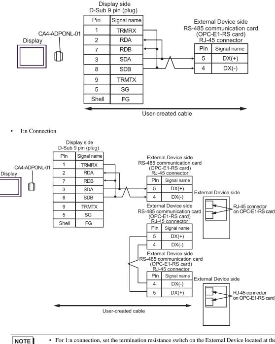
• For 1:n connection, set the termination resistance switch on the External Device located at the end to ON.
