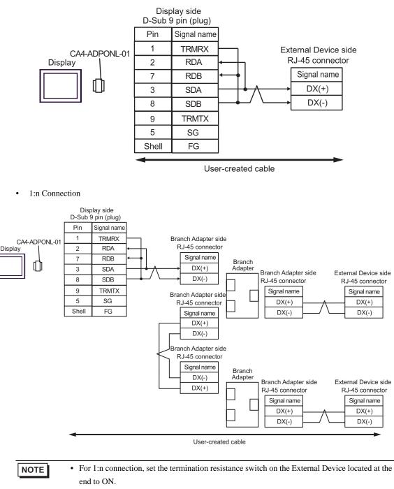
• The recommended branch adapter is the SK KOHKI's MS8-BA-JJJ.
