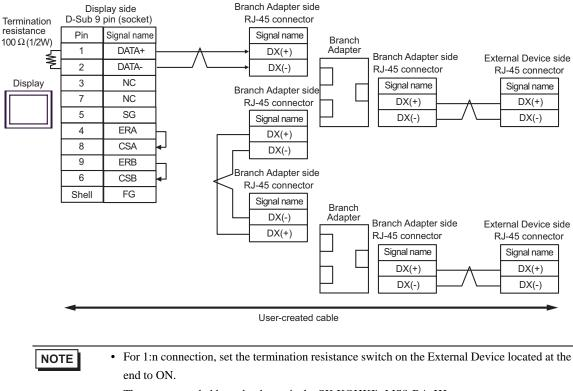
• The recommended branch adapter is the SK KOHKI's MS8-BA-JJJ.
