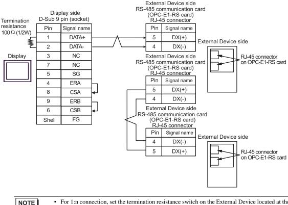
• For 1:n connection, set the termination resistance switch on the External Device located at the end to ON.
