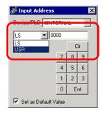
The GP's internal device [#INTERNAL], has two structured areas: the [LS] area and the [USR] are (shown below).
