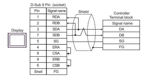
• No termination resistor is required.
