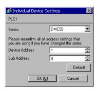
Use the ladder software (Smart Loader Package SLP-D510 V2.2.3) to configure communication settings for the External Device. Use the rotary switch on the front of the Controller to set the device address of the External Device.
