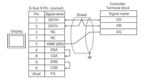
• No termination resistor is required.
