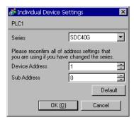
To configure communication settings for the External Device, use the PARA, ENT, DISP, Down and Up keys on the front of the Controller. You can change the communication settings only in READY mode. Switch the External Device to READY mode before setting.
