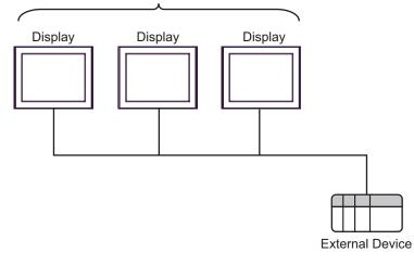
• The maximum number of connectable Displays is 16 units. However, keeping performance in consideration, the number of Displays that can be substantially used is up to 4.
