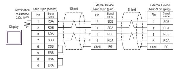
**NOTE** • When the display unit you use is an IPC, turn ON the DIP switch 6 to insert the termination resistance.
