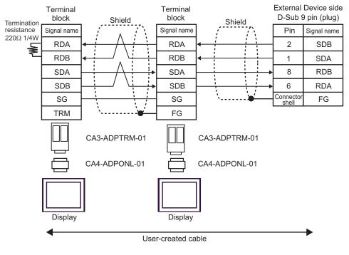
E) When using the online adapter (CA4-ADPONL-01), the multilink cable (CA3-CBLMLT-01) by Pro-face and user-created cable
