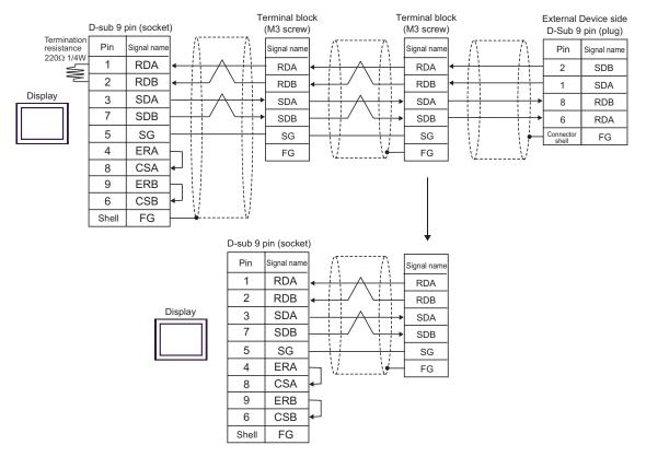
D) When using the online adapter (CA4-ADPONL-01), the connector terminal block conversion adapter (CA3-
