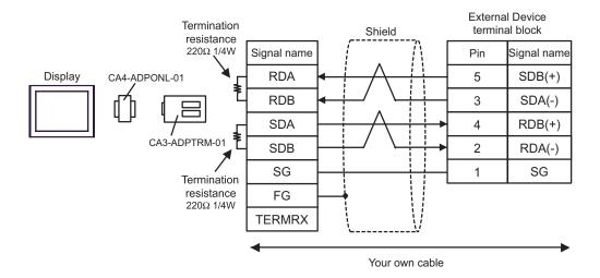
D) Cable diagram using the online adapter (CA4-ADPONL-01) by Pro-face and user-created cable
