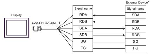
\*Turn On the termination resistance switch of the External Device, and set the operation mode to 3.
