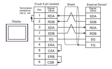
\* Turn On the termination resistance switch of the External Device, and set the operation mode to 3.
