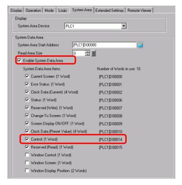
4 If you turn ON Bit 1 in the [Control: (1 Word)] address specified in step 3 while Bit 4 is OFF, the GP display unit buzzer rings.
