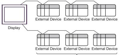
Maximum number of External Devices in Si2 series: 30 Maximum number of External Devices in CutyAxis2 series: 20 Maximum number of External Devices in CutyAxis3 series: 20
