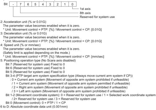
\*27 The device descriptions of Scara relative coordinate movement are shown below.
