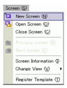
2 The [New Screen] dialog box appears. From [Screens of Type], select [Window Screens]. The [Screen] number field is filled in starting from 1. You can change this number, but it cannot be duplicated.
