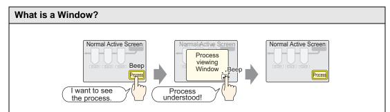
You can register occasionally viewed screens as Window screens and use a switch to show or hide the screen. Window screens are suitable for displaying reference or error handling information.
