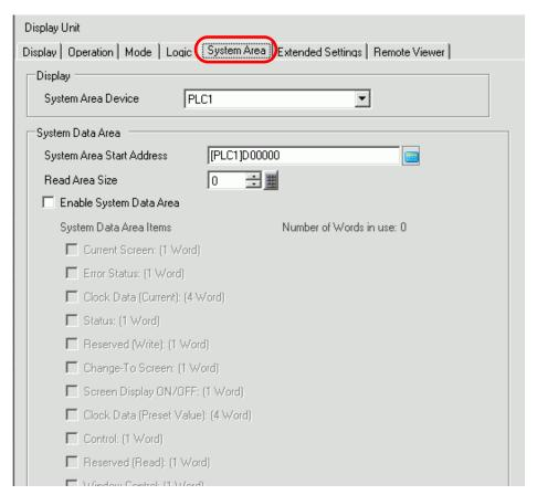
5 In [System Area Device], select the appropriate device that uses the system area. In [System Area Start Address], define the top address.
