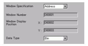
5 Click [OK]. The Window is configured according to the value stored in the address.
