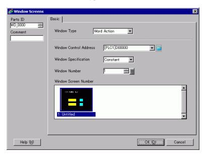
3 In [Window Control Address], set the word address (D100) that controls the window.
