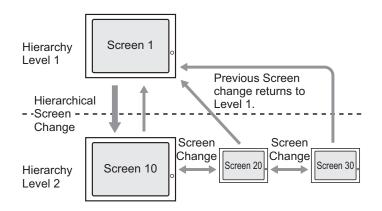
Then place a switch on Screen "10" to move up to Base Screen "1".
