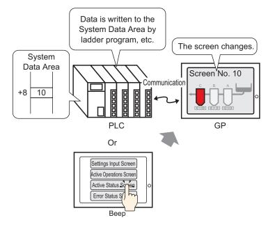
You can change screens either from a Change Screen Switch or the device/PLC.
