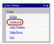
**3** Under the [Display] tab, set the [Initial Screen Number] to 1 to display this screen when the GP turns ON. This will be the first screen to be displayed when the power is ON.
