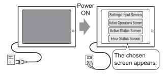
You can specify which screen is displayed when the GP power turns ON.
