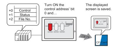
You can capture the screen displayed on the GP to a CF card. The screen capture is saved as a JPEG file (\*.jpg).
