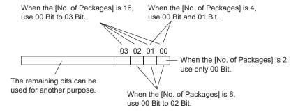
• If an undefined package is selected, the Picture Display will show nothing. For example, when the [Number of Packages] is 16, and 0 to 3 are the only packages registered, states 4 to 15 will display only the background rectangle.
