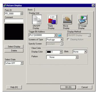
6 Under [Display Unit] select [Move Display] and in [Control Word Address] enter "D100".
