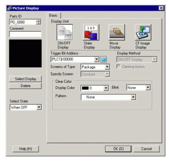
7 Under Display Type select [ON/OFF Display] and in [Trigger Bit Address] enter "M100".
