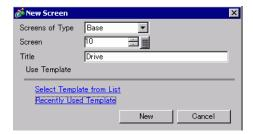
4 Create a screen to be called. Draw a rectangle the same size as the rectangle on Base 1. Set its fill color to red. When this screen is called as a Picture Display, it will affect the color in the overlapping area on the call destination screen, but will not completely obscure the original contents.
