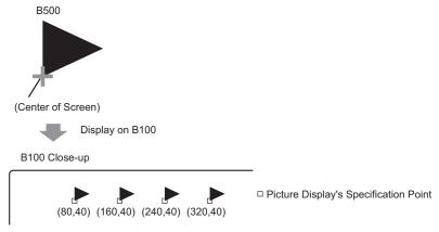
The screen to call is displayed with its center overlapping the point specified on the picture display.
