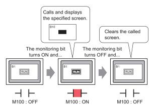
1 Create a screen on which the load operation will take place. (For example, Base1)
