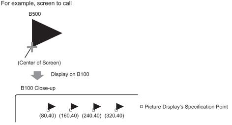
The screen to call is displayed with its center overlapping the point specified on the picture display.
