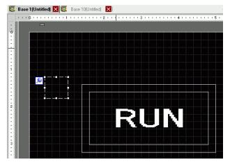
6 Double-click within the border of the Picture Display part to open the Picture Display dialog box.
