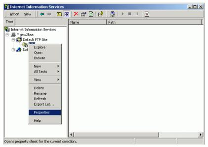
**3** Open the [FTP Site] tab, and enter the IP address of the computer in the [IP Address] field. (For example, [IP Address] 192.168.1.31)
