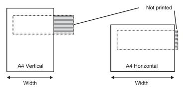
• For Screen print out on a display with a screen size larger than SVGA, see below as to whether the data fits the paper. (VGA and QVGA fit both A4 and A3 papers.)
