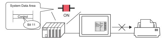
• The internal device LS14 or the device/PLC (control address) Bit 11 does not automatically turn OFF. While Bit 11 is ON, none of the print features will operate. Be sure to turn it OFF after canceling the print.
