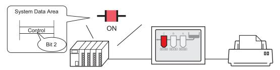
Turn ON the control address Bit 2 in the system data area allocated to a device/PLC...and
