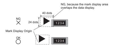
Two picture displays' positions overlap, causing an improper display.
