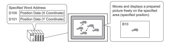
You can store the X/Y coordinates in the specified word address and load pictures from other display screens to the specified coordinates. You also move the display in a straight line between two points.
