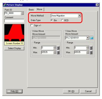
10 Under both [X-Axis Move] and [Y-Axis Move], enter the Min. and Max. Values. For example, [X-Axis Move] set Max Value to 100 and Min Value to 0, and [Y-Axis Move] Max Value to 100 and Min Value to 0.
