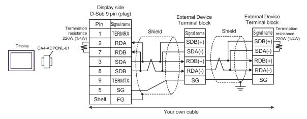
E) When using the COM port conversion adapter (CA3-ADPCOM-01), the terminal block conversion adapter (CA3-ADPTRM-01) by Pro-face and your own cable
