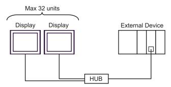
**NOTE** • The number of connectable Displays depends on the External Device. Please refer to the manual of the External Device for more details.
