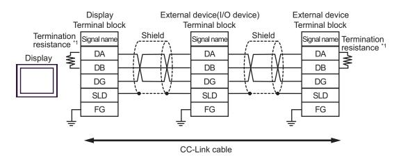
\*1 Connect the termination resistors that came with the master unit to both end devices on the data link (between DA and DB). Note that the termination resistance varies depending on the cable type.
