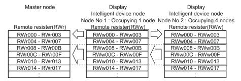
• Allocation image of the remote register (RWw) via the master station
