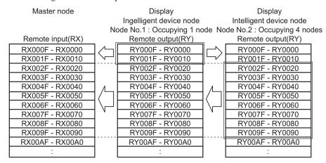
· Allocation image of the remote output via the master station
