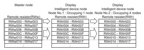
The following shows the link point specifications defined by the CC-Link Association. For CC-Link Ver.1, the extended cyclic setting is not available, and "1 time setting" is applied.
