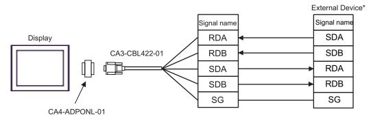
Do not connect the FG terminal of CA3-CBL422-01 to the External Device.
