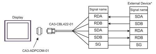
Do not connect the FG terminal of CA3-CBL422-01 to the External Device.
