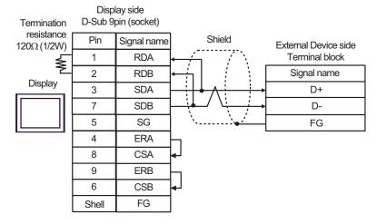
The following is a cable diagram for connecting the GP3000H series using the abovementioned External Device connection cable:
