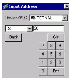
Select the device "LS", input "20" in the address, and press the "Ent" key.
