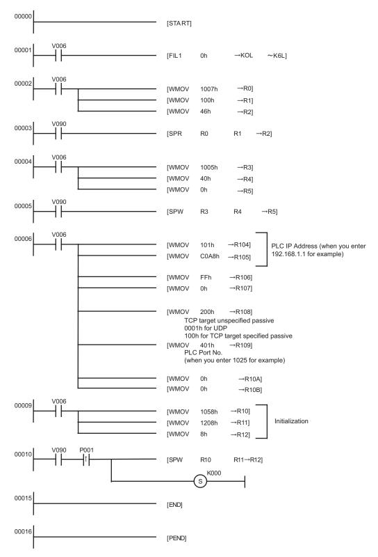
• When the communication parameter is set by both the link parameter and the ladder program, the setting by the link parameter normally is given priority. However, when you select [Initialize by Initial Sequence Program] in the link parameter setting screen, the setting by the ladder program becomes effective even if the link parameter is set.
