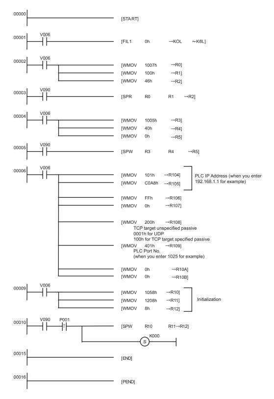
• When the communication parameter is set by both the link parameter and the ladder program, the setting by the link parameter normally is given priority. However, when you select [Initialize by Initial Sequence Program] in the link parameter setting screen, the setting by the ladder program becomes effective even if the link parameter is set.
