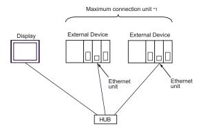
\*1 You can connect up to 32 units of External Device for UDP, and 16 units of External Device for TCP at the same time.
