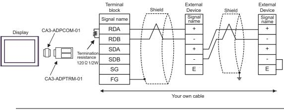
IMPORTANT • Use the lead wire to connect between "-" terminal and "E" terminal in the External Device which terminates the connection.
