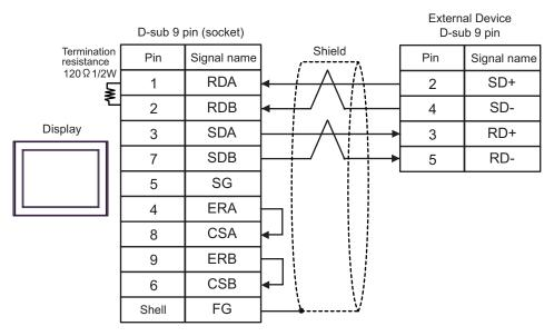
C) When using the online adapter (CA4-ADPONL-01), the terminal block conversion adapter (CA3-ADPTRM-01) by Pro-face and your own cable
