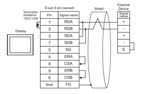
IMPORTANT • Use the lead wire to connect between "-" terminal and "E" terminal in the External Device which terminates the connection.
