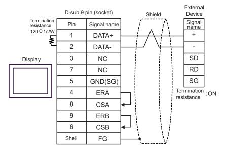
**NOTE** • Use the DIP switch in the communication cassette to set the termination resistance. Set SW1-1 of the External Device to ON.
