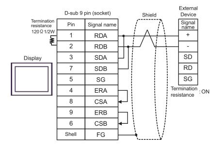
• Use the DIP switch in the communication cassette to set the termination resistance. Set SW1-1 of the External Device to ON.
