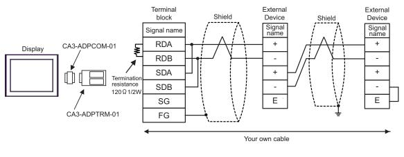
• Use the lead wire to connect between "-" terminal and "E" terminal in the External Device which terminates the connection.
