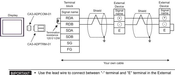
· Use the lead wire to connect between "-" terminal and "E" terminal in the External Device which terminates the connection.
