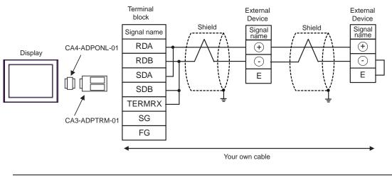
IMPORTANT • Use the lead wire to connect between "-" terminal and "E" terminal in the External Device which terminates the connection.
