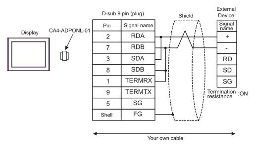
• Use the DIP switch in the communication cassette to set the termination resistance. Set SW1-1 of the External Device to ON.
