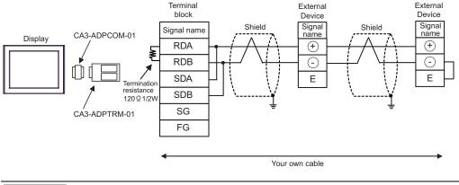
IMPORTANT • Use the lead wire to connect between "-" terminal and "E" terminal in the External Device which terminates the connection.
