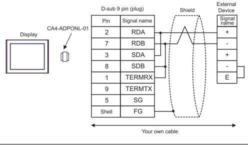
IMPORTANT • Use the lead wire to connect between "-" terminal and "E" terminal in the External Device which terminates the connection.
