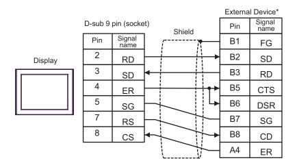
\* Set the operation mode on the External Device interface to 1.
