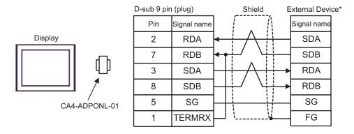
\* Turn On the termination resistance switch of the External Device, and set the operation mode to 3.
