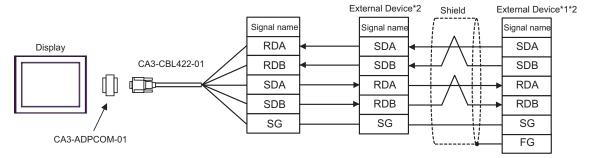
Do not connect the FG terminal of CA3-CBL422-01 to the External Device.
