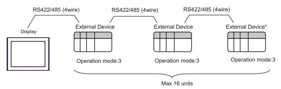
\* Turn ON the termination resistance switch on the interface which terminates the RS422 connection.
