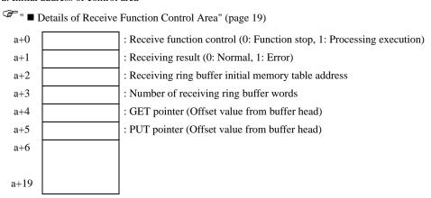
Receiving buffer that stores receive data is defined by using this Receive Function Control Area. In general, Display sets this definition immediately after the start.
