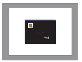
[Window Mode]: [Window Screen] [Specify Display Position] none Displayed centered in 800X600 resolution.
