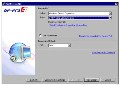
**3** Click [Communication Settings] to set up the communication format and other settings. The set up process is the same as steps 6 to 7 in 5.2.2 Setup Procedure.
