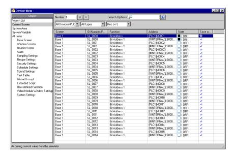
6 In the Device View, set the screen number from [Number] to switch the address display screen.
